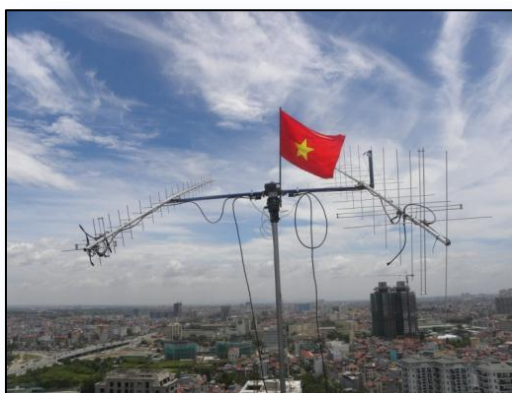
FIGURE 34: FSPACE TEAM BUILDING GROUND STATION FOR COMMUNICATION WITH LOW EARTH ORBITING SATELLITE, VIET NAM
