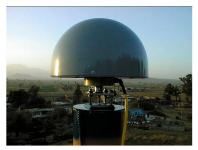
Figure 5-2. GPS Sensor for Monitoring Tectonic Movements. Credit: USGS
