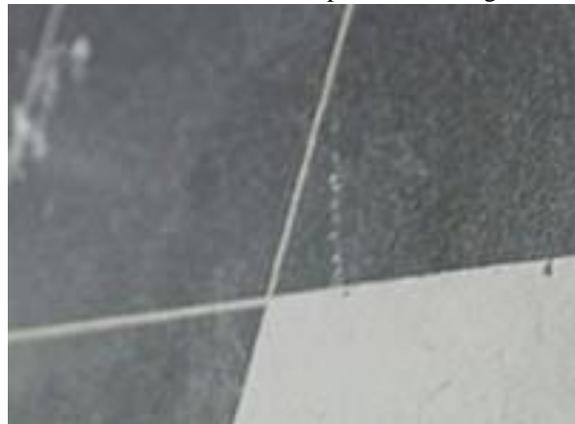
Figure 7: Sample of laser etched slate [22]. Significant change in albedo is evident, while digital measurement yield a maximum difference of 34 % to 75 % in brightness.
